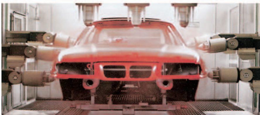
Laquering spraying system with lac-robot apparatus
